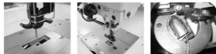
Extra heavy duty type feeding mechanism and extra large speed shuttle hook make it possible to stitch extra heavy duty material easily.
